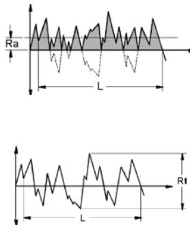
Surface roughness may also be expressed in terms of maximum roughness, depth or the distance between the peak and the base line measurement over the sampling length. **Maximum roughness** is denoted **R<sub>t</sub>**.
