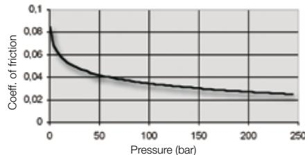
The dry friction of typical seal materials rubbing on a smooth, dry seal surface may be anything from  $\mu=0.4\div 1$ . For lubricated surfaces the range is much lower, for example,  $\mu=0.02\div 0.10$ . This is particularly true in the case of elastomers. Fabric materials and impregnated fabrics show similar values of " $\mu$ " but usually with less variation, for example  $\mu=0.04\div 0.08$  for lubricated conditions.
